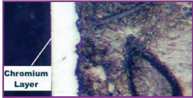
Photo micrograph of chromium-plated G25HP cast iron Originally published Nov. 2015, Industrial Heating “Ion/Plasma Nitriding Improves Die Life”
