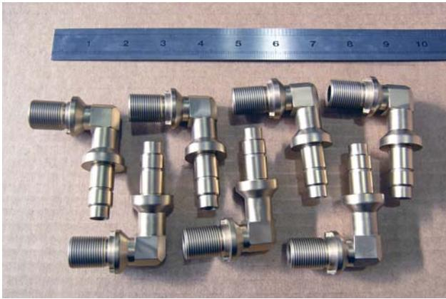
**Fig. 3. Plasma-nitrided aircraft hydraulic components for steering system made of the  $\alpha+\beta$  titanium alloys**
