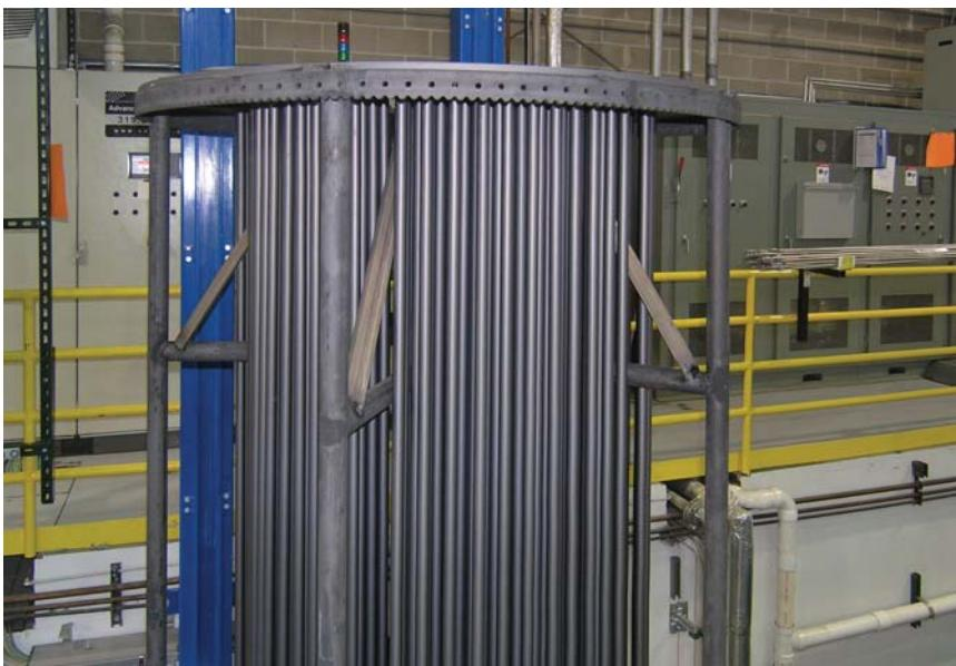
**Fig. 7. Long, low-alloy steel shafts used for hydraulic cylinder rods after gas nitrocarburizing with post oxidizing**
