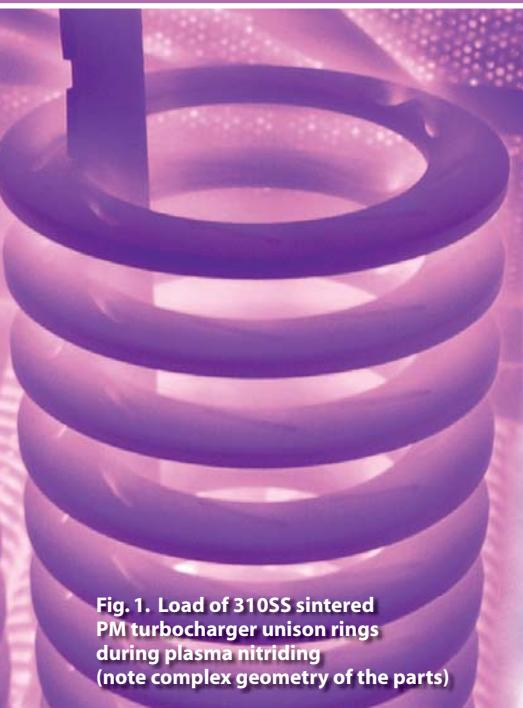
**Fig. 1. Load of 310SS sintered PM turbocharger unison rings during plasma nitriding (note complex geometry of the parts)**
