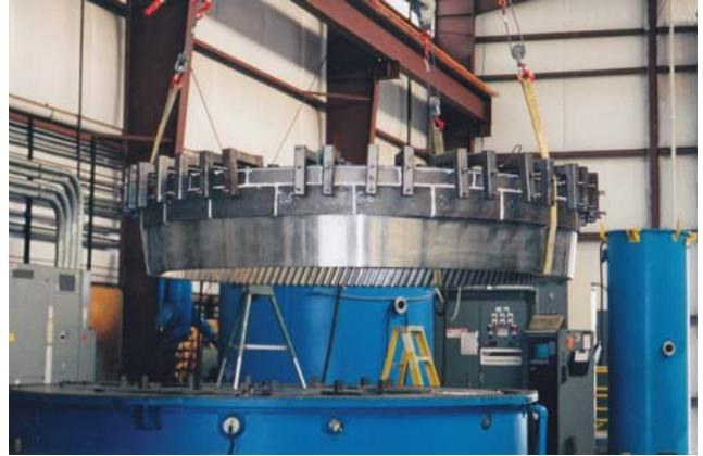
**Fig. 4. Large internal 4340 steel gear for power energy application being loaded into the plasma-nitriding vessel (note extensive mechanical masking on the outside of the gear)**
