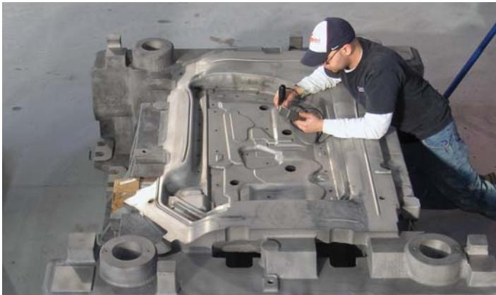
**Fig. 5. Cast iron automotive stamping dies after plasma nitriding**
